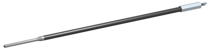
Figure 3: 5-hole probe
